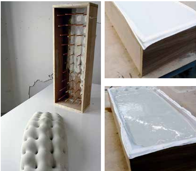
MachineHistories Fabric Form Work 1. An experiment in casting using material properties and gravity as a form finding technique. Materials: Hydrocal Gypsum, Spandex, Plywood and pencils
