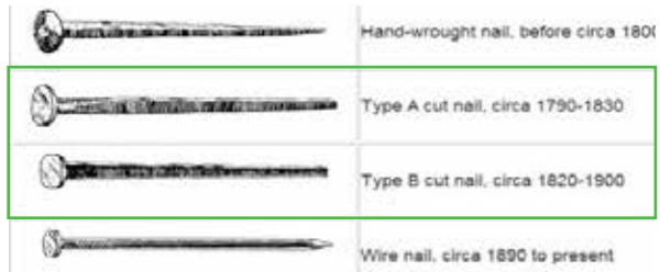
Examples of machine cut (or square) nails
