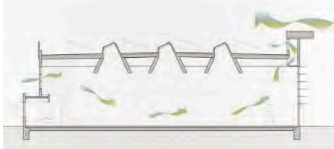
Mode 2 ■ Swing Season. Outside air quantity varies to provide coolin, and fresh air. Wind chimney only.
