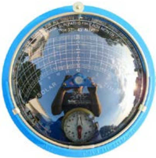
Solar Pathfinder - The Solar Pathfinder has been the standard in the solar industry for solar site analysis for decades. Its panoramic reflection of the site instantly provides a full year of accurate solar/shade data, making it the instrument of choice.
