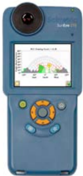
SunEye™ - The Solmetric SunEye™ is a hand held electronic device that allows users to instantly assess total potential solar energy given the shading of a particular site. Identifying the shading pattern early in the process reduces the expense of system and home design and improves the efficiency of the final system or house.
