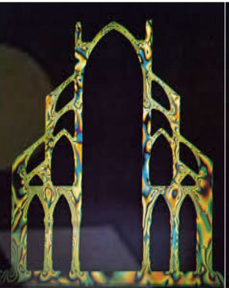
R. Mark. Force visualization on Gothic Cathedral using polarized light and plexiglass ('70s)
