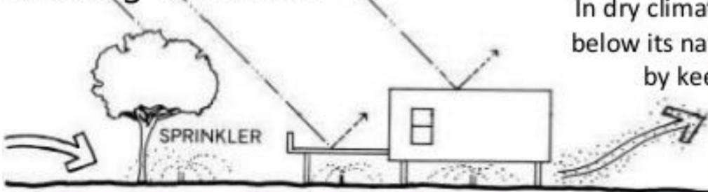
In dry climates, soil can be cooled significantly below its natural temperature by shading it and by keeping it wet for evaporative cooling.
