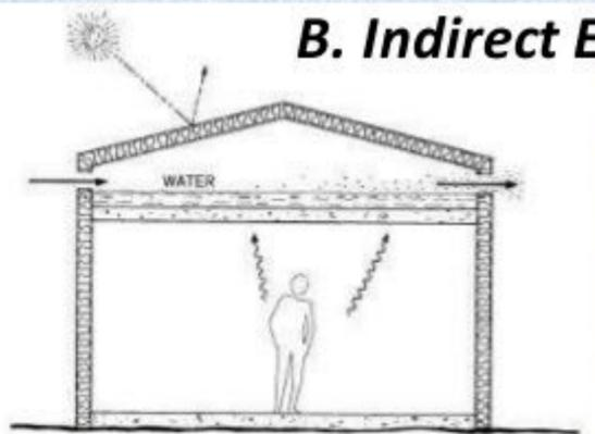
This indirect evaporative cooling system uses a roof pond. Note no humidity is added to the indoors.
